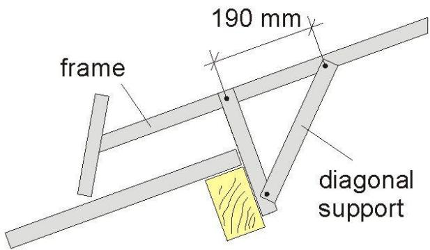
4. Now the diagonal support is attached and fixed to both the support and the frame with two SX5 drill screws (see sketch).
