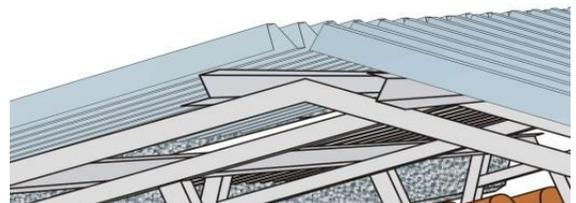
Place the domes and attach them to all Z purlins in each second lower flange with SX5 stainless steel drill screws. Then the light panels are fixed on all purlins to every 2nd chord with SX5 stainless steel self-drilling screws. **Never** mount the light panels the other way round because of the coextrusion!
