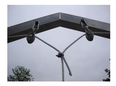
13. Finally, the chain is attached to the end of the traction rope with a rope clamp.
