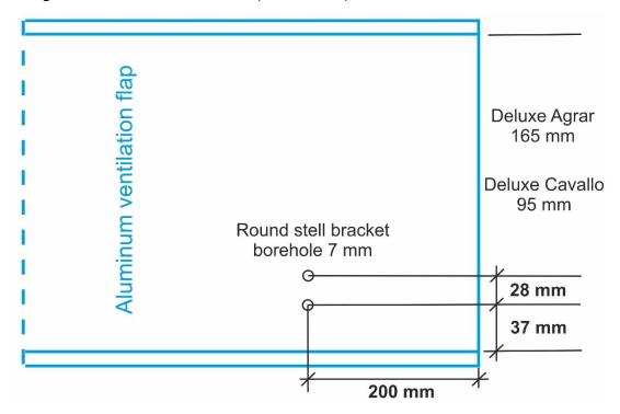
7. Fasten the aluminum ventilation flaps to the rotary tube using round steel brackets with a rectangular double hole washer and 25 mm washers and nuts. The flaps should be aligned when they are closed.
