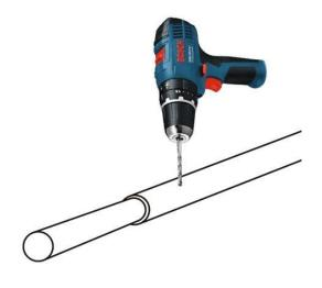
5. If the ridge is longer than 30 m, an additional locking lever must be installed. The individual sections are separated next to a support. At this support, two eye brackets are placed side by side and rotary tube is separated between the eyelets. Thus, the individual sections of max. 30 m may be adjusted independently.
