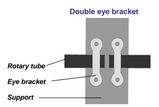
6. The holes in the aluminum ventilation flaps to accommodate the round steel brackets are made with a 7 mm iron drill. The lower hole is 37 mm and the upper 65 mm from the lower edging of the ventilation flap. There is 200 mm on each side from the lateral outer edge to the center of the hole (see sketch).
