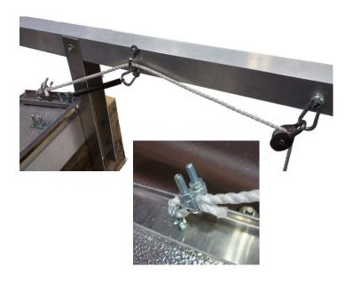
12. On the other side of the ridge, also guide the traction rope through the pulley and eye bracket and fasten it to the eyelet of the ventilation flap with a rope clamp.
