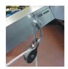
10. The eye bracket is attached to the frame with SX 5 drilling screws for the rope guide.
