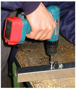
Fasten the eye brackets with the SX 5 drilling screws without pre-drilling!
