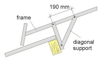
5. Put Al-Z-Pfetten Al-Z-purlins on the frame, according to sketch, and fix each support with two SX5 drill screws. The overlap of the purlins is 120 mm and is located exactly on a frame. Pay attention to the correct size of ridge and the number of the row of purlins per side.
