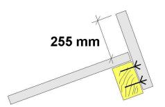
2. Stretch a cord and align the other supports and also fasten them with two resp. three drill screws. The support spacing for the »Deluxe Agrar Type Hall « MLL 60 to 200 is 1440 mm (center to center supports) or 960 mm for the MLL 225 to 400. The spacing is necessary to be observed.
